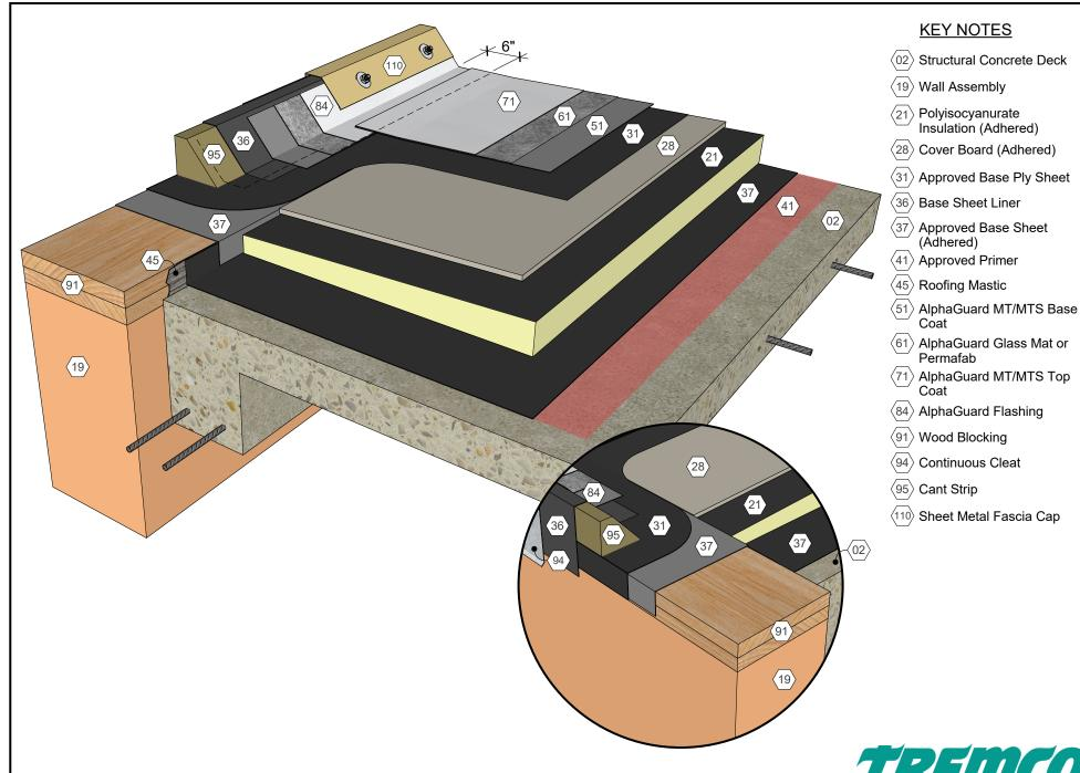
AlphaGuard® MT/MTS Plus Raised Perimeter Edge, Temp. Roof, Structural Concrete Deck Detail 32022
