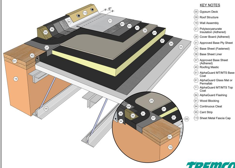
AlphaGuard® MT/MTS Plus Raised Perimeter Edge, Temp. Roof, Gypsum Deck Detail 32025
